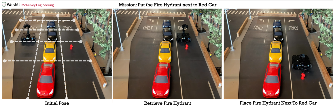
Figure 2: Evaluation in a physical environment with OOD scenarios sampled from \mathcal{D}' . The robot receives the NL instruction ‘put the fire hydrant next to the red car.’ The left panel shows the 3 \times 5 grid abstraction used for planning, where each cell represents a discrete navigation step. Using this representation, the LLM planner generates \tau directing the robot to turn, move to the hydrant, pick it up, move to the red car, and place the hydrant next to it.
