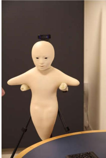
**Fig. 1.** The Telenoid™ tele-operated robot for robotic tele-presence
