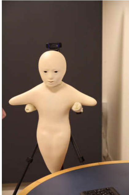
Fig. 1. The Telenoid™ tele-operated robot for robotic tele-presence
