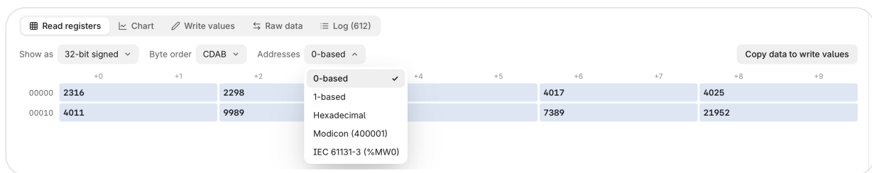
Figure 9. Holding registers read as 32-bit values.
