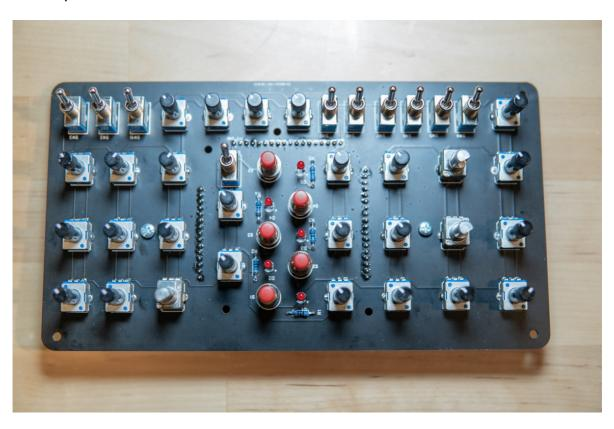
**STEP14**Place the panel and screw the pots and switches
