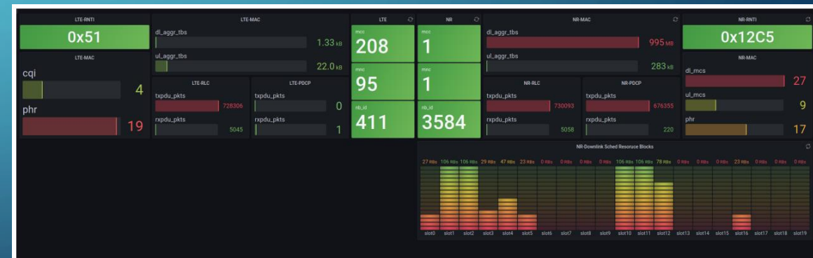
Figure: srsRAN 4G eNodeB and OAI 5G gNodeB monitoring PDCP, RLC and MAC SM
