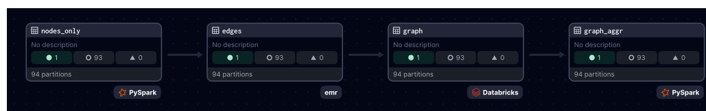
Figure 2: Detailed dagster pipeline showcasing how execution environments can be chosen as needed between local, EMR and DBR.
