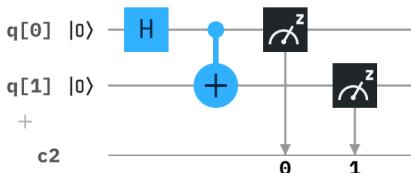
Circuits are using quantum bits (starting in state  $|0\rangle$  grouped in quantum registers), classical register for measurement reading, and gates applied to qubits from left to right in time sequence.
