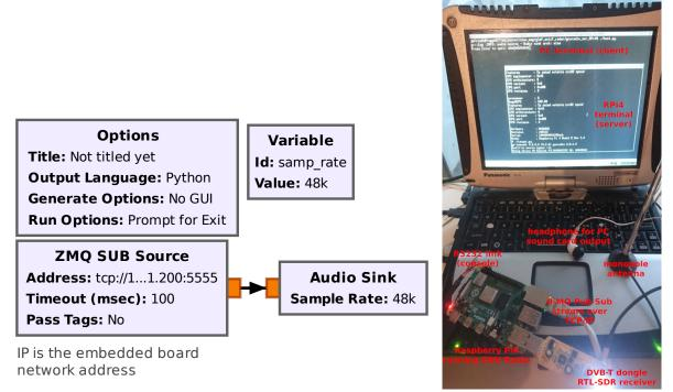
Left: client flowchart, fetching a 0-MQ subscribe datastream and feeding the sound card of the host PC. Right: experimental testbed, with the RPi4 connected though virtual serial port and Ethernet to the laptop PC. The RPi4 collects an I/Q stream from the DVB-T dongle tuned to an FM-broadcast station, streams the demodulated audio flow to
