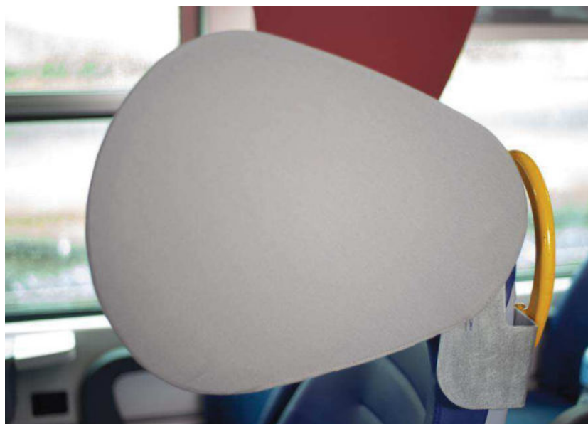
Figure 12. Representative images of a liner in PES fabric.
