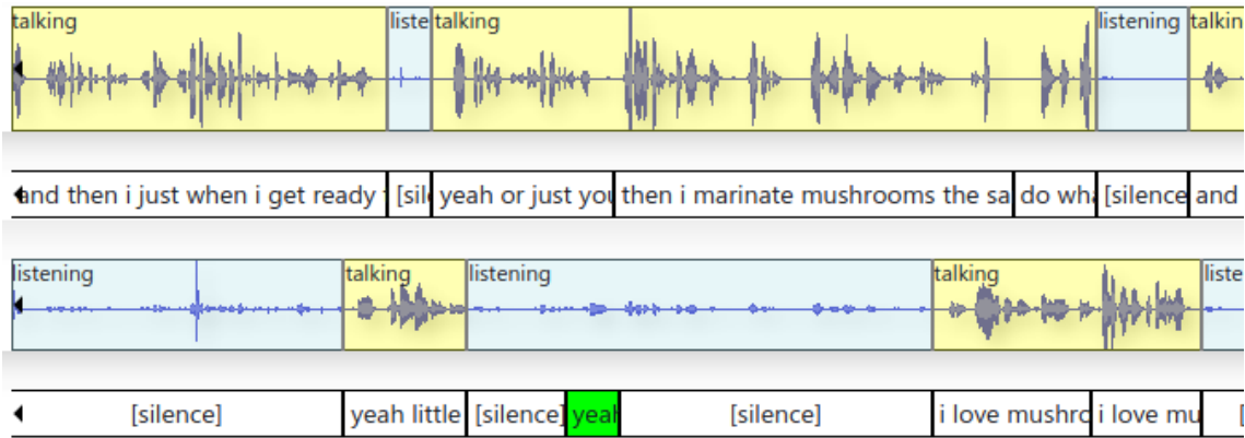
Figure 4.10: A short audio segment showing the automatically classified talking and listening areas. Note that a backchannel from Speaker B in the middle (“yeah”) does not classify that area as speaking. At the end both people talk at the same time, so Speaker B needs to repeat themselves.
