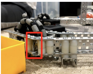
Boxed c channels for rigidity around gussets.
