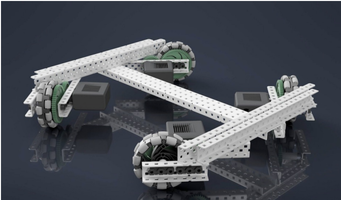
Design option without the use of 45 degree gussets where the angles are built using the offset of 2 outer c channels
