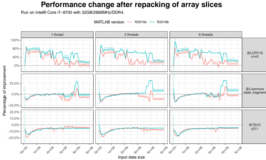
Fig. 6: Result of applying repacking of array slices. Not every computation benefits from the transformation (TSVC/s211).
