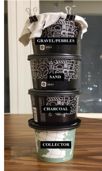
Figure 5: Biofilter model with removable containers
