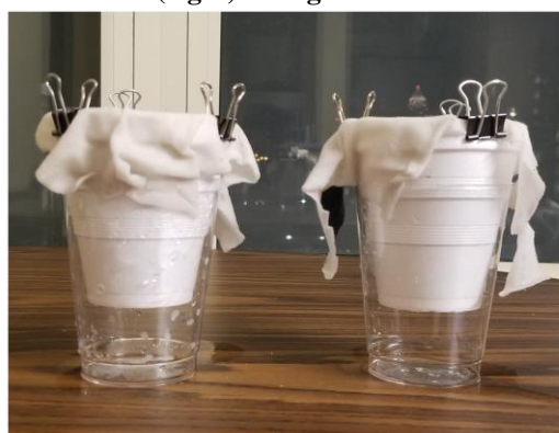
Figure 2: Small test filters with pebbles, sand and cloth (left), and pebbles, sand, charcoal and cloth (right) configurations
