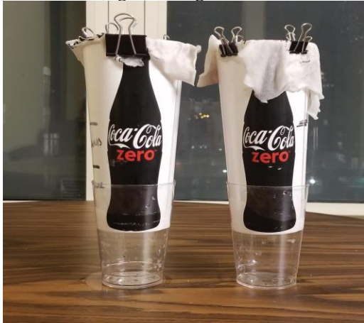
Figure 3: Large test filters with pebbles, sand and cloth (left), and pebbles, sand, charcoal and cloth (right) configurations
