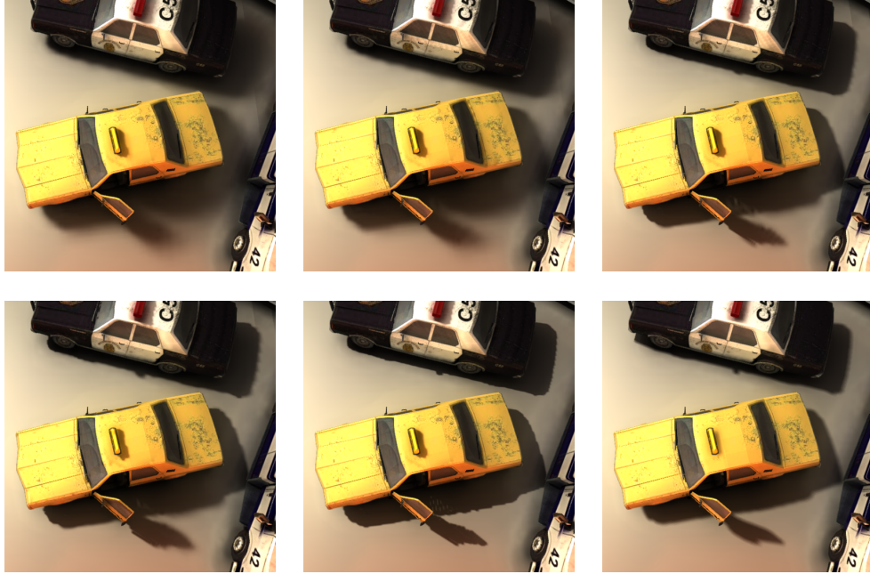
Figure 17. Cone traced direct shadows with different cone apertures. In reading direction, the shadows in the first three pictures are traced with cone apertures of 9^\circ , 6^\circ and 3^\circ . Note that the individual voxels become noticeable at 6^\circ near the siren of the police car. On the third picture one can notice light leaking near the taxi door, due to thin voxelization with non-conservative triangle rasterization and a large step size. On the bottom left picture the conservative rasterization is enabled, yet some leaking remains due to the thin voxelization. On the fifth picture the aperture is set to 0^\circ and the last picture shows shadow mapping with percentage closer filtering for comparison. See Table 5 for time measurements.
