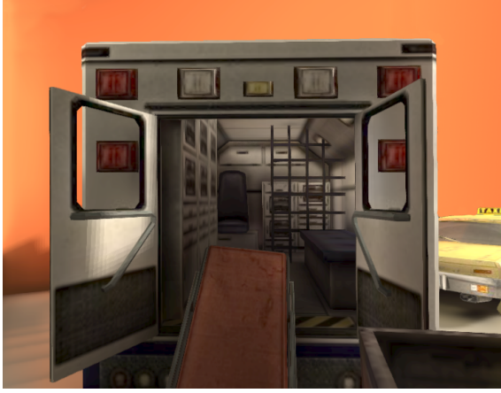
Figure 12. Light leaking inside the ambulance. Light leaking may occur when voxels are sampled that are averaged over both lit and unlit regions. This is in particular a result of the wide cones which are used for sampling the diffuse indirect light. The expected result is a dark interior as there are no light sources inside the ambulance.
