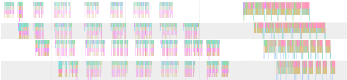
Figure 6.3: Analysis of the PyTorch Bottleneck profiling tool on a GPipe application using ResNet-18 with CIFAR-10 on 4 GPUs with 8 micro-batches. First the forward pass is executed, then the backward pass. Only compute-related workload is shown.
