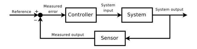
The most common type of algorithmic controller is the *PID controller*. Over 95% of industrial applications and a wide range of biological systems employ elements of PID
