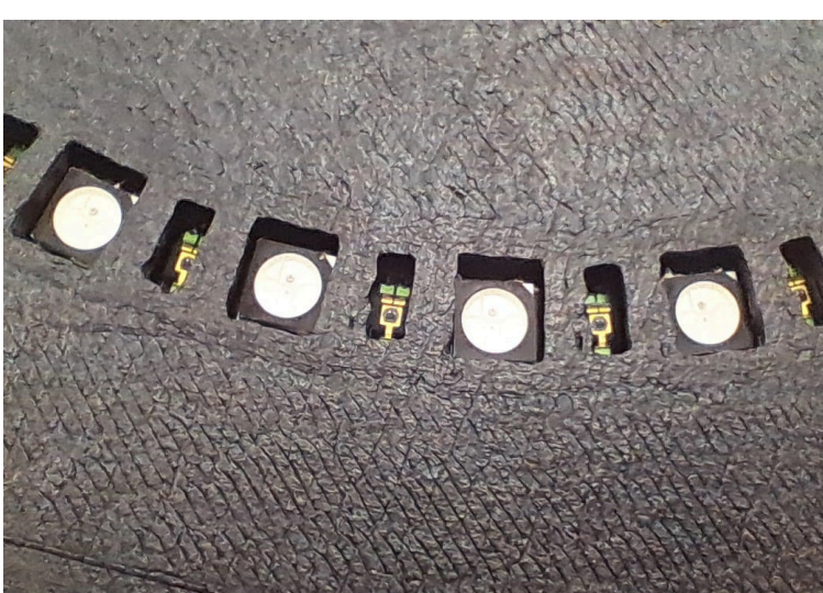
Fig. 4 - Reflectance sensors on the bottom board.
