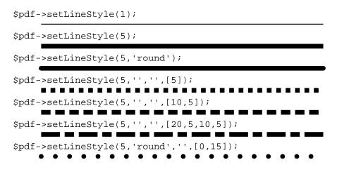
Note that the code shown with each of these lines is just the line style command, the drawing of each line also requires a **line** command, which is not shown.
