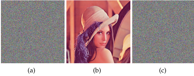
Fig. 15. We observe the effect of Trojan-infected AES to recover the secret key. (a) Encrypted image, (b) Decrypted image with recovered key. (c) Decrypted image with random key.
