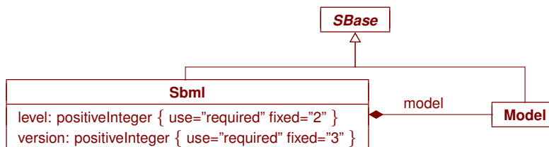
Figure 4: A more complex example definition drawing on the concepts introduced so far in this section. Both Sbml and Model are derived from SBase ; further, Sbml contains a single Model object named model . Note the constraints on the values of the attributes in Sbml ; they are enclosed in braces and written in XML Schema language. The particular constraints here state that both the level and version attributes must be present, and that the values are fixed as indicated.
