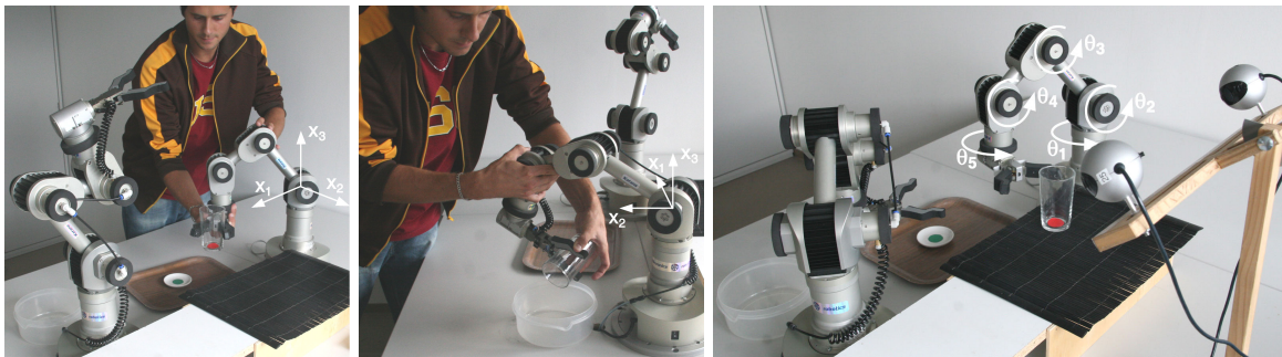
Figure 1: Kinesthetic demonstrations of the two tasks considered in this experiment, namely grasping and placing a glass on a coaster ( left ), and grasping and emptying a glass ( middle ). Right : Reproduction of the skill by the two robots, during which the initial positions of the objects are tracked by a stereoscopic vision system.
