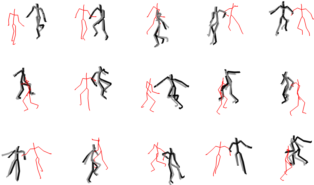
Figure 6: Example of TP-MFA to encode and retrieve full-body dancing motion from [36]. Here, the motion of one of the two partners ( D=94 ) is retrieved by adapting it online to the motion of the other partner. In the model, the red stick figure (in thin line) is the frame of reference and the gray stick figure (in thick line) is the motion encoded in TP-MFA. The black stick figure (in thick line) shows the motion regenerated with TP-MFA and Gaussian mixture regression, based on the observation of the red stick figure. For 12 Gaussian components ( K=12 ) and a subspace of 2 dimensions ( d=2 ) encoding a motion of 94 dimensions, the total number of parameters in TP-MFA is 4511. The corresponding number of parameters in a TP-GMM with full covariances would be 54719. We can see that TP-MFA generates a smooth and natural movement similar to the original dance.
