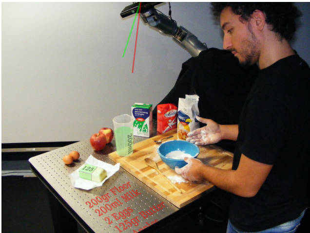
Fig. 10 Illustrative scenario of a robot assistant in the kitchen. Cooking often requires the use of both hands. With hands in flour, the user could not use a standard external interface to easily follow the recipe while doing the task. Here, a possible implementation could be to project information on the required amount of milk and butter and the list of ingredients without interrupting the task (namely, by having the text oriented towards his sight).
