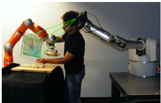
Fig. 11 Illustrative scenario of an interactive skill analysis process. A section of the 3D flow field related to the task is projected on the board, while the user moves the planar surface in the manipulator's workspace.
