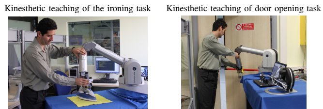
Fig. 3. Teaching the positional profiles of the ironing task and door opening task.
