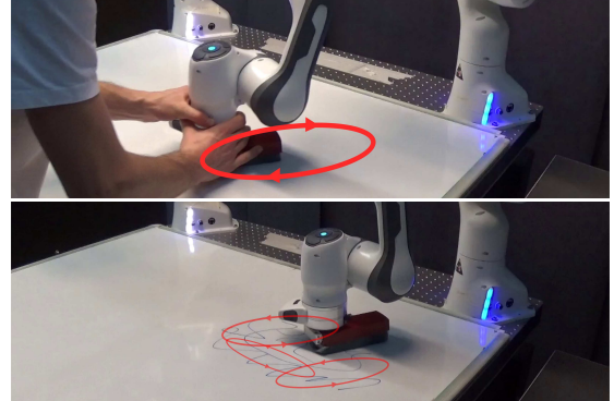
Fig. 1: Rhythmic tasks such as wiping need to be demonstrated in few demonstrations ( top ), while the robot should extract the important motion features (e.g. amplitude, frequency and phase) and generalize it in a consistent, safe manner ( bottom ).
