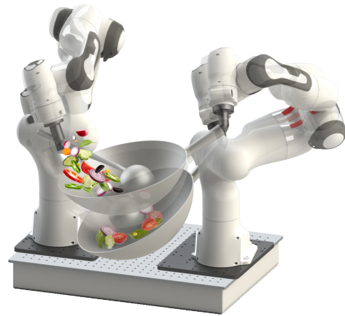
Fig. 1. Robot stir-fry is a non-prehensile manipulation of semi-fluid objects which requires highly dynamic movements and continuous bimanual coordination in a long time series.
