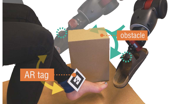
Figure 18: Variant (a) of the task to put on a shoe while facing an obstacle. The obstacle is kept static. The robot learns to avoid it from the right or the left side based on what is more convenient given the position of the user's foot.
