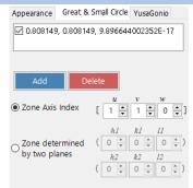
Draws large circles and small circles. Specify by the index of the zone axis or the index of the two crystal planes.
