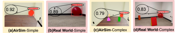
Fig. 4. Preprocessing on drone view provides sphere detection in simulation and real world environments.
