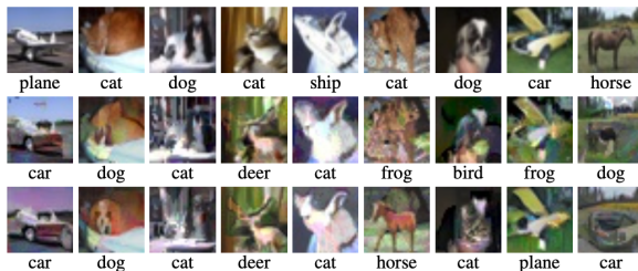
Figure 2: Attack images built for adversarially trained models look like the class into which they get misclassified. We display the last 9 CIFAR-10 clean validation images (top row) and their adversarial examples built for a 7-PGD adversarially trained (middle) and our “free” trained (bottom) models.
