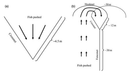
Figure 1. Top view of crossnet (a) and multiple-net (b) designs. The dashed hooknet represents the reset on the opposite crossnet end.
