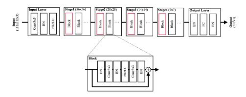
Figure 2. Block diagram of the network we used in this challenge. The channel-size for each *Stage* was set to 64, 128, 256, and 512, respectively. In the first *Blocks* (denoted in red rectangles), we set the stride of 2 for each of the first *Conv3x3* layers.
