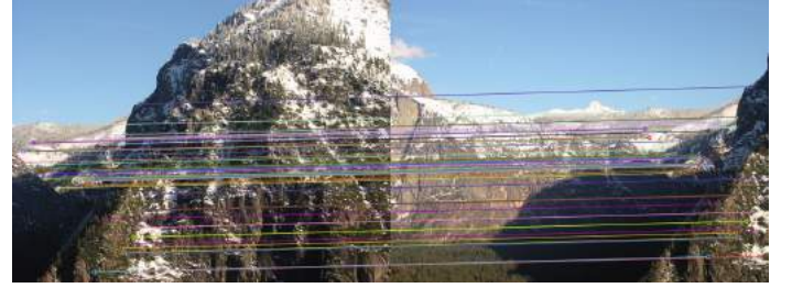
Fig. 3. SIFT feature matching using Brute force method
