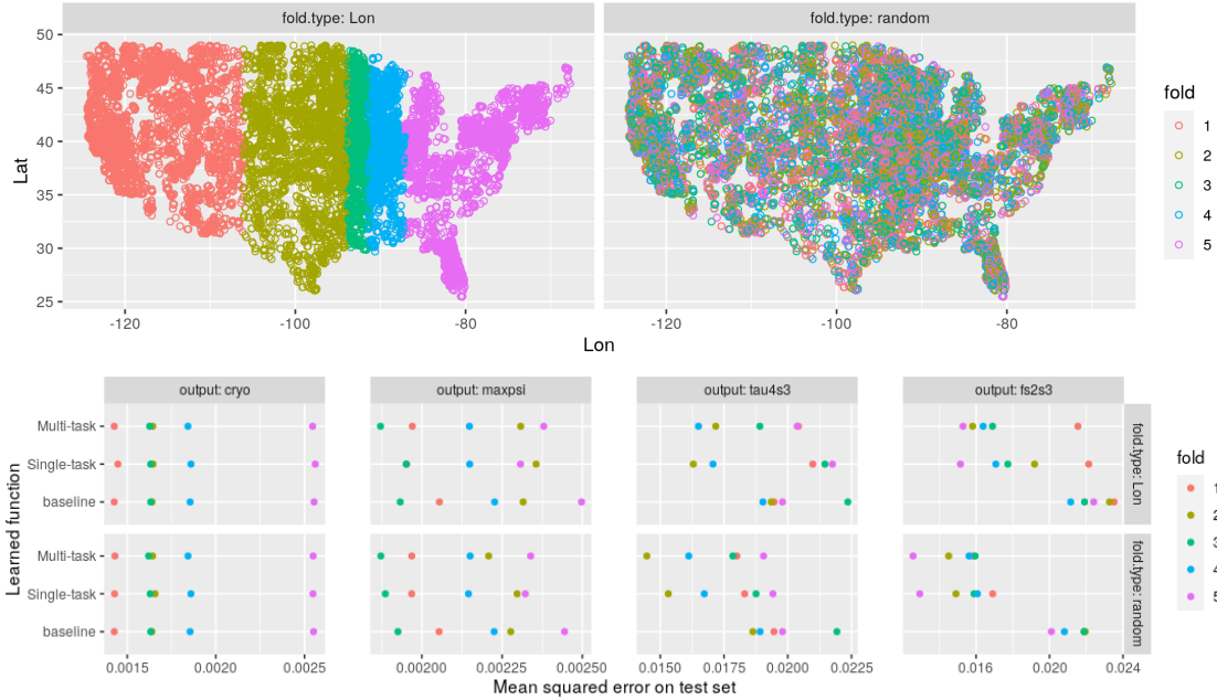
Figure 5: Cross-validation for estimating error rates on machine learning algorithms that predict earth system model parameters. Top: fold IDs were assigned to each observation using longitude (left) or randomly (right). Bottom: prediction error for four of the 25 outputs. Please see [Tao et al., 2020] for meanings of abbreviations (cryo, maxpsi, tau4s3, fs2s3).
