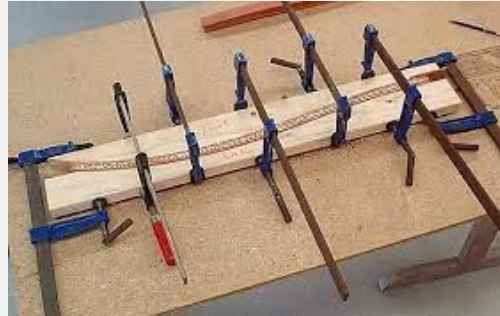
Holding device - Holds and lines up material
