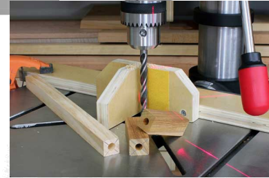
Drilling Jigs - Helps locate the hole accurately and quickly
