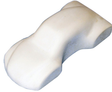
Former - Soft material is pulled over the shape
