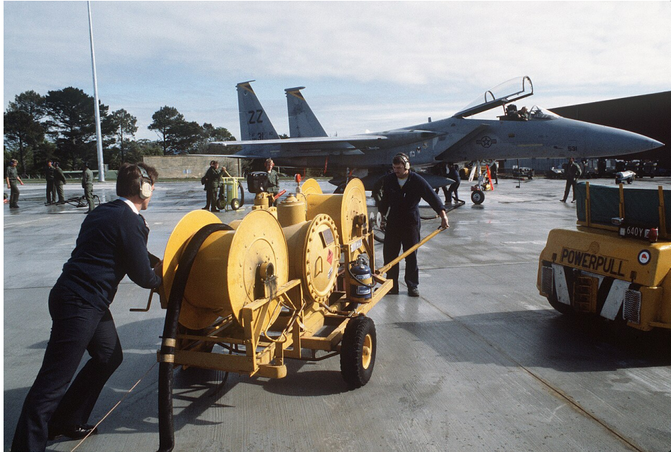
Photo: Department of Defense. American Forces Information Service. Defense Visual Information Center. 1994 — Public domain — via Wikimedia Commons (Maintenance_crewmen_push_a_refueling_hose_reel_to_an_F-15A_Eagle_aircraft_of_the_12th_Tactical_Fighter_Squadron_
