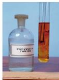
▲ Figure 12.7 Bromine displaces iodine from potassium iodide solution.
