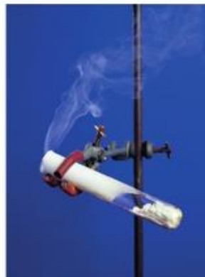
Figure 21.2 Heating ammonium chloride
