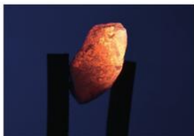
▲ Figure 5.16 A glowing piece of limestone. Limestone is impure calcium carbonate – it decomposes when heated to form calcium oxide (quicklime) and carbon dioxide. This is a thermal decomposition reaction.
