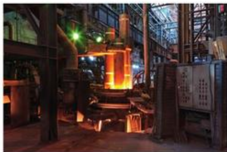
▲ Figure 8.31 Three graphite electrodes glow red hot after their removal from an electric arc furnace used to produce steel.
