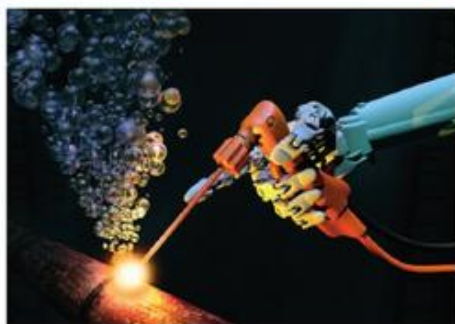
▲ Figure 19.4 The burning of hydrogen is used in oxy-hydrogen cutting equipment underwater.
