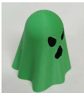
0.08 mm layer height print time: 1h 19m
