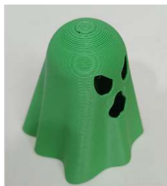
0.28 mm layer height print time: 28m 27s
