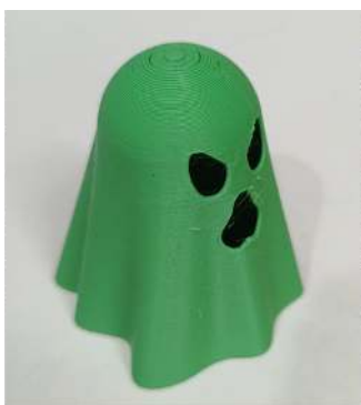
0.2 mm layer height print time: 36m 14s
