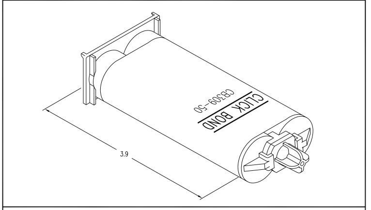
CB309 EPOXY ADHESIVE IN DUAL PACK CARTRIDGE
