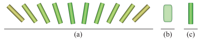
Figure 1: Two types of mean tensors for (a) 10 linear anisotropic tensors with the same eigenvalues (0.7, 0.15, 0.15) but different eigenvectors. (b) is the Euclidean mean and (c) is the ensemble mean calculated according to Equation (3).
