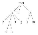
Only those nodes that form a path from the root to one of the nodes of the tree can be in memory at a time. Thus, for the above example, the root node and nodes a, c and e can be in memory simultaneously, or the root node, and nodes k and m can be loaded at the same time, but not the nodes a, g and h because they do not form a path from the root to one of the nodes.
