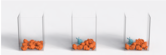
Fig. 34. We drop 10 bunnies in a container with different settings to show how different matrix sizes generated in Hessian computation affect the total memory consumption. Left: all 10 bunnies are soft. Middle: 9 bunnies are soft and 1 bunny is controlled by affine body (colored light blue). Right: same as middle, but we turn on the optimization where we separate the generation of inner Hessian and Jacobian matrices, which reduces the memory size.
