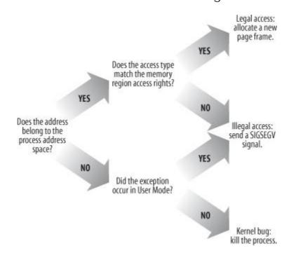
Figure 9-4. Overall scheme for the Page Fault handler
