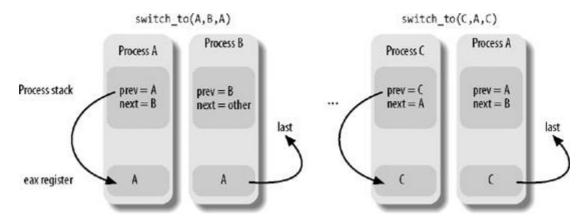
The switch\_to macro is coded in extended inline assembly language that makes for rather complex reading: in fact, the code refers to registers by means of a special positional notation that allows the compiler to freely choose the general-purpose registers to be used. Rather than follow the cumbersome extended inline assembly language, we'll describe what the switch\_to macro typically does on an 80x86 microprocessor by using standard assembly language:
