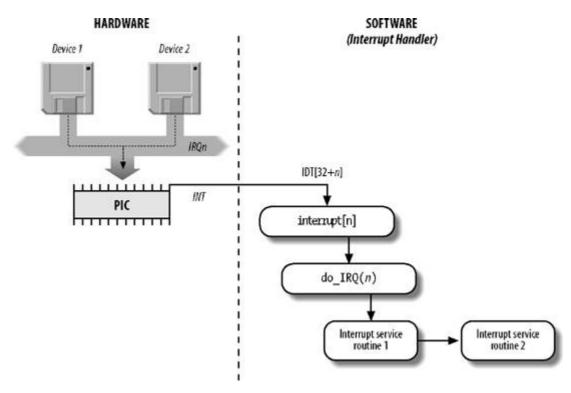
Figure 4-4. I/O interrupt handling
