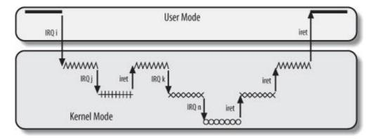
The price to pay for allowing nested kernel control paths is that an interrupt handler must never block, that is, no process switch can take place until an interrupt handler is running. In fact, all the data needed to resume a nested kernel control path is stored in the Kernel Mode stack, which is tightly bound to the current process.
