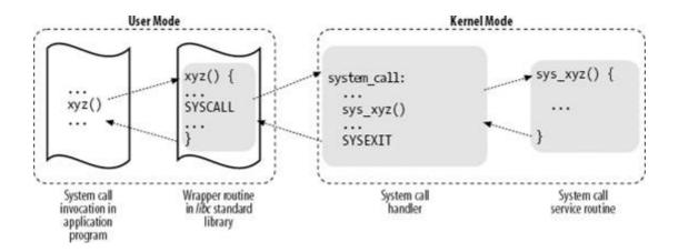
To associate each system call number with its corresponding service routine, the kernel uses a system call dispatch table, which is stored in the  $sys_call_table$  array and has  $NR_syscalls$  entries (289 in the Linux 2.6.11 kernel). The  $n^{th}$  entry contains the service routine address of the system call having number n.
