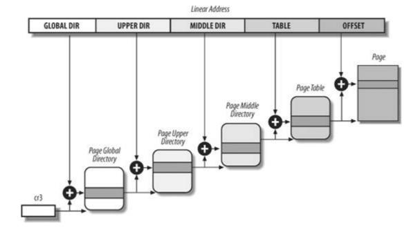
For 32-bit architectures with the Physical Address Extension enabled, three paging levels are used. The Linux's Page Global Directory corresponds to the  $80 \times 86$ 's Page Directory Pointer Table, the Page Upper Directory is eliminated, the Page Middle Directory corresponds to the  $80 \times 86$ 's Page Directory, and the Linux's Page Table corresponds to the  $80 \times 86$ 's Page Table.
