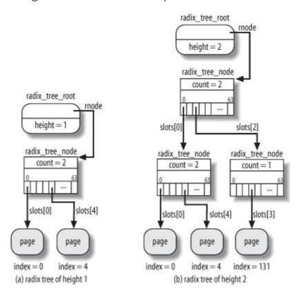
Figure 15-1. Two examples of a radix tree
