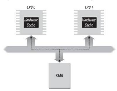
Figure 2-11. The caches in a dual processor
