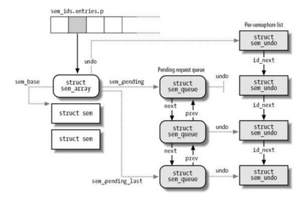
Formally, the array stores pointers to kern\_ipc\_perm data structures, but each structure is simply the first field of the sem\_array data structure. All fields of the sem\_array data structure are shown in Table 19-10.
