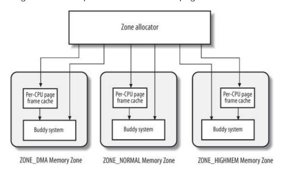
Figure 8-2. Components of the zoned page frame allocator
