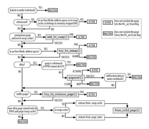
To reclaim an anonymous page, the page must be added to the swap cache, and a new slot in a swap area must be reserved for it; see the section "Swapping" later in this chapter for details.
