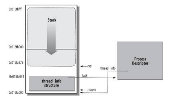
The esp register is the CPU stack pointer, which is used to address the stack's top location. On 80x86 systems, the stack starts at the end and grows toward the beginning of the memory area. Right after switching from User Mode to Kernel Mode, the kernel stack of a process is always empty, and therefore the esp register points to the byte immediately following the stack.
