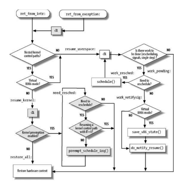
The flow diagram gives a rough idea of the steps required to resume the execution of an interrupted program. Now we will go into detail by discussing the assembly language code.
