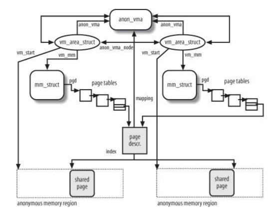
the section "The clone(), fork(), and vfork() System Calls" in Chapter 3); the kernel simply inserts the anonymous memory region of the second process in the doubly linked circular list of the anon\_vma data structure pointed to by the anon\_vma field of the first process's memory region. Therefore, any anon\_vma's list typically includes memory regions owned by different processes. [\*]
