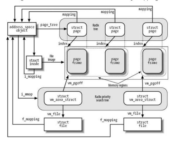
Figure 16-2. Data structures for file memory mapping
