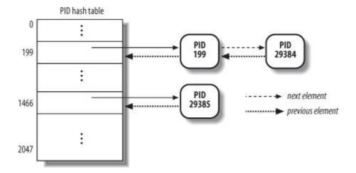
The PID hash tables' data structures solve all these problems, because they allow the definition of a list of processes for any PID number included in a hash table. The core data structure is an array of four pid structures embedded in the pids field of the process descriptor; the fields of the pid structure are shown in Table 3-6.
