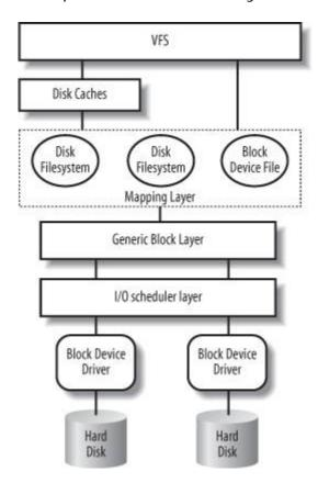
is the upper layer of the block device handling architecture, and it provides a common file model adopted by all filesystems supported by Linux. We have described at length the VFS layer in <a href="Chapter 12"><u>Chapter 12</u></a>.
