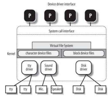
Some user programs (P) wish to operate on hardware devices. They make requests to the kernel using the usual file-related system calls and the device files normally found in the <code>/dev</code> directory. Actually, the device files are the user-visible portion of the device driver interface. Each device file refers to a specific device driver, which is invoked by the kernel to perform the requested operation on the hardware component.
