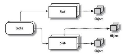
Figure 8-3. The slab allocator components
