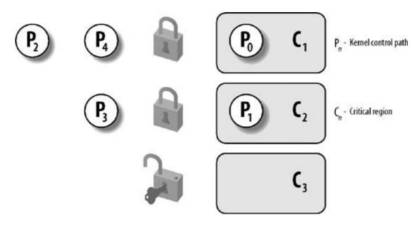
*Spin locks* are a special kind of lock designed to work in a multiprocessor environment. If the kernel control path finds the spin lock "open," it acquires the lock and continues its execution. Conversely, if the kernel control path finds the lock "closed" by a kernel control path running on another CPU, it "spins" around, repeatedly executing a tight instruction loop, until the lock is released.
