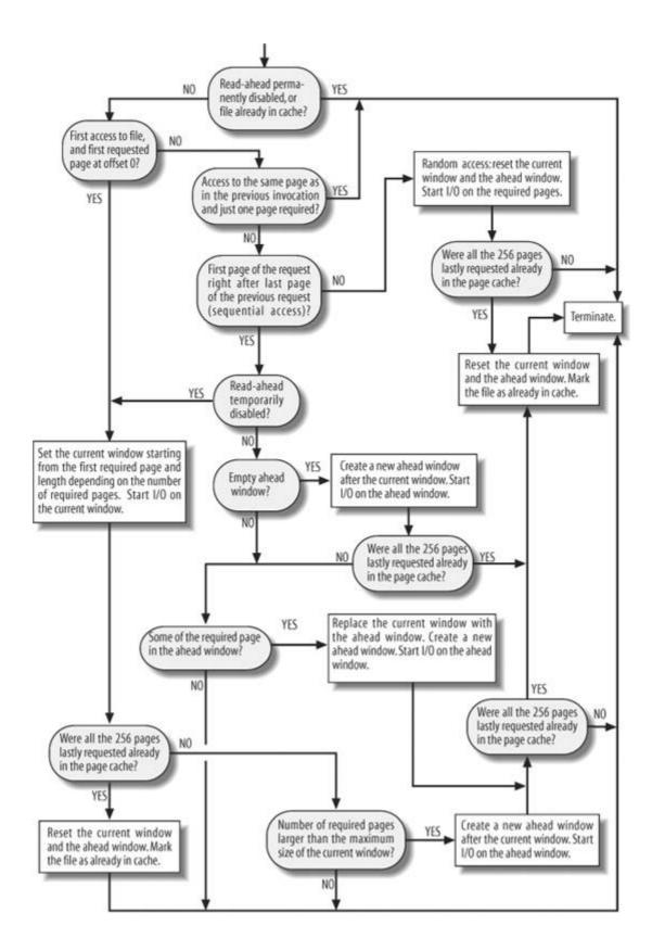
Every time page\_cache\_readahead( ) creates a new window, it starts the read operations for the included pages. In order to read a chunk of pages, page\_cache\_readahead( ) invokes the blockable\_page\_cache\_readahead( ) function. To reduce kernel overhead, the latter function adopts the following clever features:
