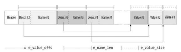
Figure 18-2. Layout of a block containing extended attributes
