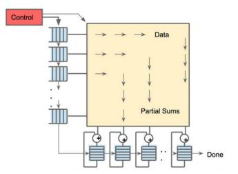
Hardware pipelining of steps in matrix-multiply. Figure courtesy Google.
