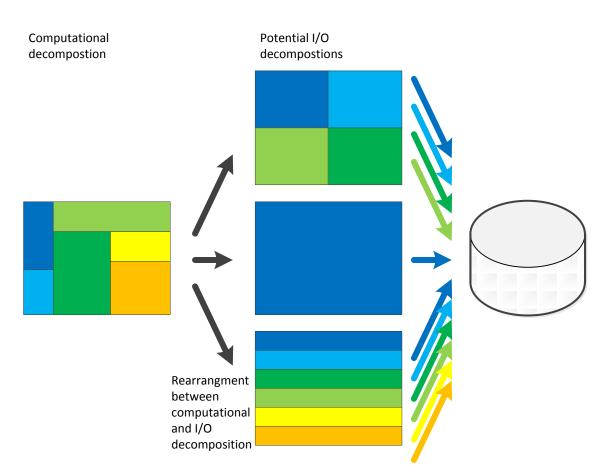
Figure 3: Separation between computational and I/O decomposition in PIO (the different colours represent the computed processes on which the respective data resides)
