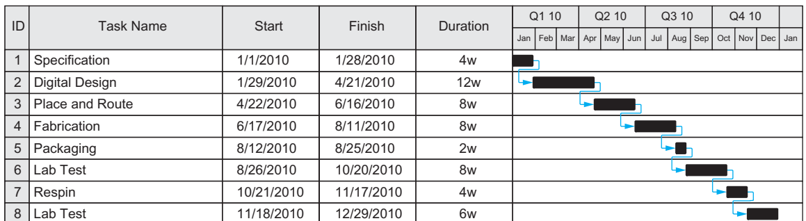
FIGURE 14.28 Gantt chart for simple chip
