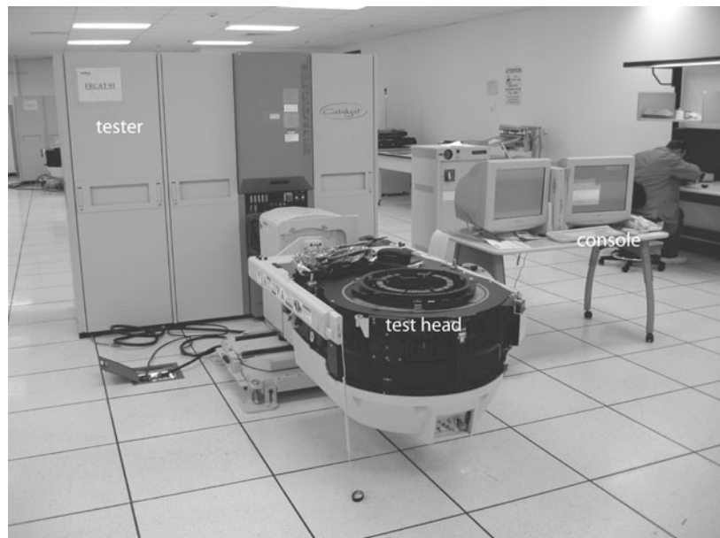
FIGURE 15.3 The Teradyne Catalyst: A typical production tester (Photo: John Haddy, Cisco Systems.)
