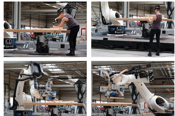
Figure 5: The human and the robot are fixing the timber slats into position using different tools.
