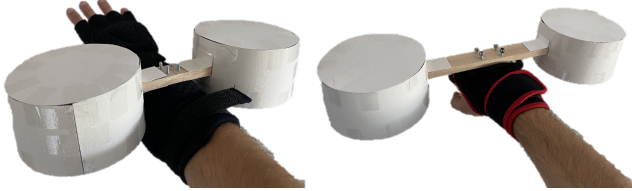
Figure 2: The paper mockup used in our form factor pre-study. Left/right: attached to the wrist/hand.
