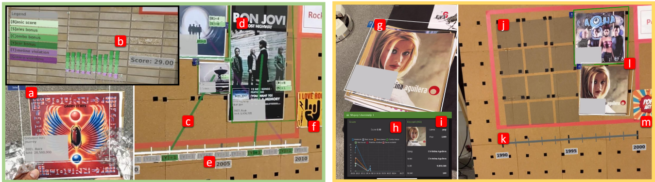
Figure 5: Visualizations for the Head condition (HoloLens 2) on the left and the Tab condition (iPad Pro) on the right. Situated information is not available in the Tab condition; only visual cues which are necessary to perform the task are kept in 3D. For example, the tracked border of the exhibit is highlighted to provide feedback on the successful recognition of objects. (a) A tracked exhibit in Head shows detail information on the bottom left and the “select” button on the top left, while (g) the tracked exhibit in Tab does not present detail information; (i) the detail information in Tab is shown as a 2D panel. (b) Head shows the color-coded score chart, with the legend to the left and the current score to the right, on a nearby wall, while (h) Tab shows it as part of the panel mentioned above. (c) Head introduces the leader lines from the exhibits to the corresponding year, while the leader lines are missing in Tab. (d) Head shows bonus scores for an exhibit placed on the wall, while (i) Tab shows only the border without additional information. (e) The timeline in Head indicates the year bonus (green “Y+1”), (k) which is missing in Tab. (f, m) The “recalibration” markers for the pop and rock wall. Similarly, the (j) grid is also the same under both conditions.
