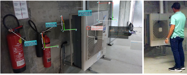
Fig. 9. (left) AR view of the automatically generated visualization, consisting of an info-panel on the left, with a leader line to the sensor, and a time-series graph on the right. (right) A user wearing a HoloLens looking at an instrumented ventilator.
